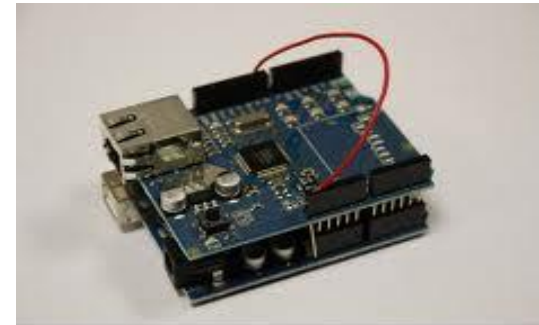
Arduino Ethernet Shield Pinout http://community.arduino.cc/tutorials/001-ethernet-shield-pinout/ The ethernet shield will crash if the RESET pin is not hooked up (to something). In the above hardware configuration the RESET pin of the shield is hooked up to Digital [9] as an output. It goes to LOW to reset the shield then back to HIGH before every ethernet connection it makes.
