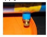
remove. You can do it by opening the valve that is in the bottom side of air tank. Before you do it you must switch off the compressor or all humidifier.
