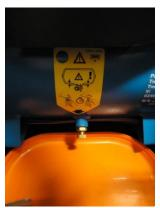
**Emptying of air tank**- the air tank in the compressor can collect the water. The water must be remove. You can do it by opening the valve that is in the bottom side of air tank. Before you do it you must switch off the compressor or all humidifier. **Connecting a computer to microcontroller.** You have to remove the white lid. You must switch off the power supply (On/Off button) and then connect the usb cable.
